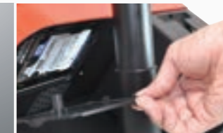
Easily Removable HDD (1 Screw)
